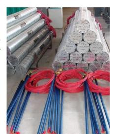
The galvanized steel canisters form part of the anode and will be consumed in service. Due to the sacrificial effect between the canister and the coke, it is advised that storage time be kept to a minimum so as to avoid corrosion and perforation of the canister.
