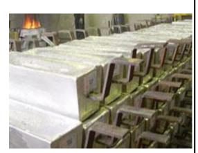
**Anode life** – As with any other anodes, anode life depends on the current output of the anode. The more current output provided by the anode, the shorter the anode's life. Therefore, it is important to consider a number of factors when selecting the type and quality of anodes. These factors include electrolyte resistivity, structure surface area, coating integrity, temperature, and design life.
