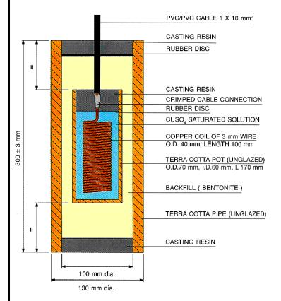
ArmREF-DC type of permanent reference electrode is recommended for applications where the soil would be dry for long terms of operation period such as CP installation in desert, and also is recommended type for external CP monitoring of storage tank bottom cathodic protection applications.
