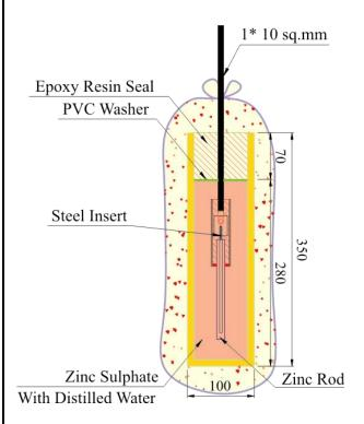
Each Reference electrodes have been completed within suitable length of continues  $1 \times 10$  Sq.mm CU/XLPE/PVC Black Cable tail depending to the application requirements.
